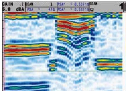
Laminar defects in metallic or composite materials are easily viewed in the Phased-Array mode.
