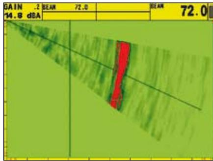
Scribe line cracking is easier to locate and quantify with Phasor XS.
