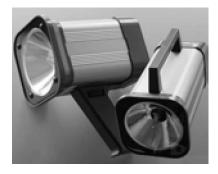
Series DT-311& 315N stroboscopes can either be hand-operated or mounted on a tripod, and can be used to observe fast repeated motions as well as to determine RPM or rate of machinery components. Not only continuous motions of materials, but also processes, which are normally impossible to observe due to their high rate, can be visualised.
