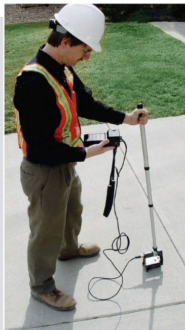
The CTG gauge can be used overhead, on a wall, or attach the telescoping pole for use on flatwork and hard to reach places
