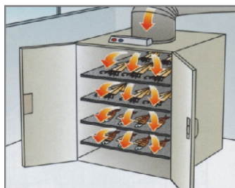
■ Airflow Control inside of Drying Oven
